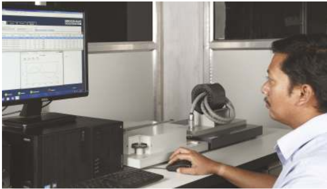
Epstein test setup from Brockhaus, Germany
