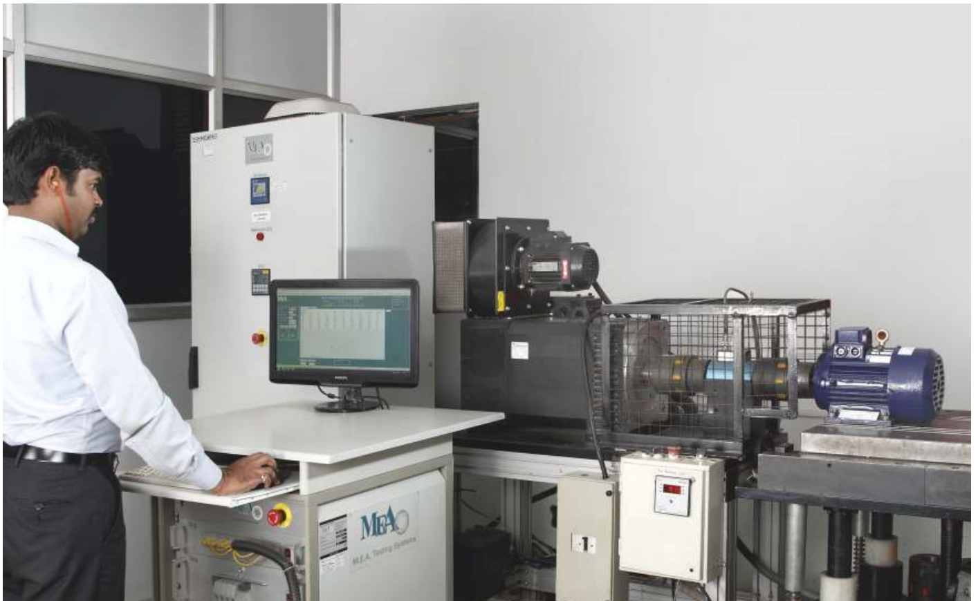
Dynamometer testing for LT motors
